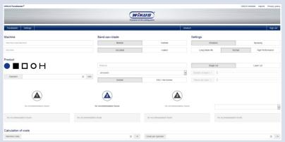
In particular, ParaMaster<sup>®</sup> supports with the choice of band saw blade and identifying the cutting parameters, whilst also determining the cutting costs at the same time. If the user accepts the recommendation of the ParaMaster<sup>®</sup> results, he can significantly reduce the costs per cut.
