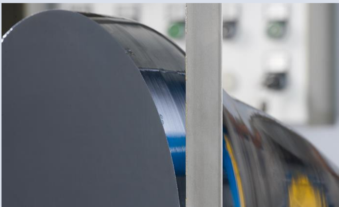
Figure 2: Sawing silicon with segmented diamond coating
