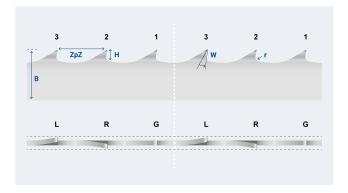
B = band width, tpi = teeth per inch, H = tooth height, W = cutting angle, r = radius, L = left, R = right, G = straight
