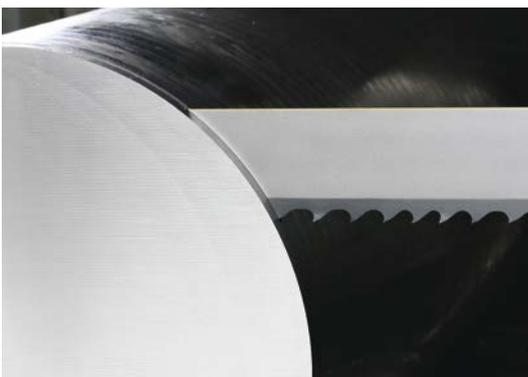
Another innovation is the SELEKTA® GS PREMIUM M42, which is used for the cutting of solid materials and metals up to 1400 N/mm<sup>2</sup> tensile strength.
